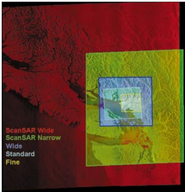
FIGURE 4.5: Area coverage of RADARSAT beam modes
