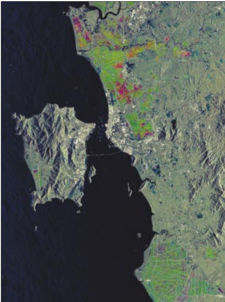
Coastal zone mapping of Penang, Malaysia using a multitemporal merge of three RADARSAT scenes. RADARSAT data © Canadian Space Agency/Agence spatiale canadienne 1996, 1997. Received by the Canada Centre for Remote Sensing. Processed and distributed by RADARSAT International.
