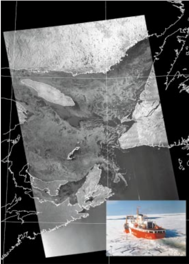
FIGURE 4.3: Ship routing using RADARSAT ScanSAR Wide beam mode
